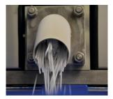
Quick change of dry ice stick size thanks to extrusion dies fixed with only 4 bolts
