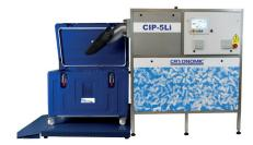
CIP5Li pelletiser with integrated scale and CIC550 dry ice container
