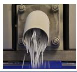
Quick change of dry ice stick size thanks to extrusion dies fixed with only 4 bolts
