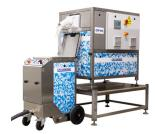
Dry ice blaster feeded directly with dry ice from a CIP5Si pelletiser
